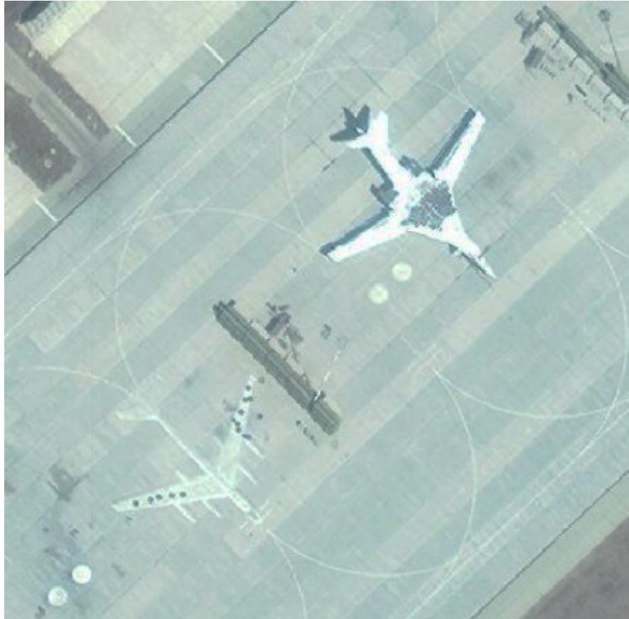
Figure 17 Russians on the Engels airbase painted bomber silhouettes on the tarmac. However, thanks to the shadow of a real plane on the right we can definitely say the left one is fake.
