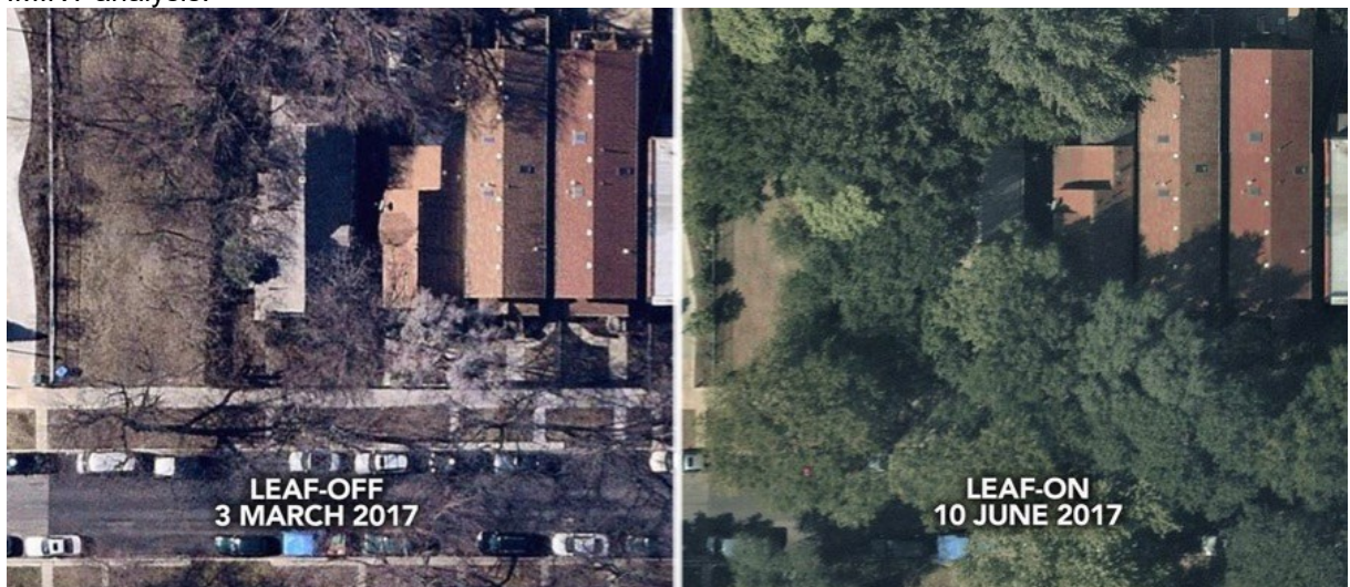
Figure 18 Season can have a big impact, e.g., with leaf off conditions we can see underneath structures.
